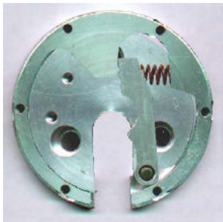
View of clamp assembly with rear cover removed. Note that the spring is green in most applications (Bolts not shown)
